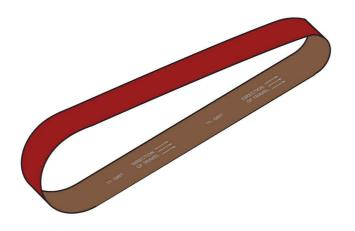
Ceramic: A synthetic grain formulated to withstand extreme pressures and dissipate heat. The synthetic chrystals fracture to continually expose sharp edges for aggressive cutting action.
